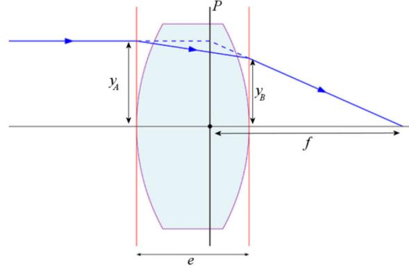
$y_B$  is the distance between the ray and the principal axis at point B on the second surface.
