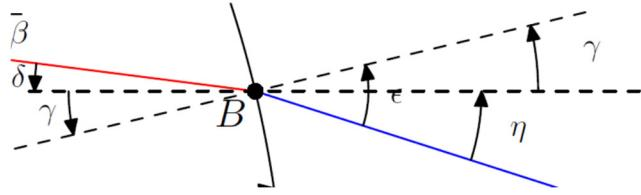
The angle  $\varepsilon$  is the angle on the refracted ray. Thus, according to the law of refraction
