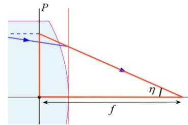
Now, we must make the link between the angle  $\eta$  and  $y_A$ . To achieve this, we will travel along the ray to get to the first surface. We will work with the following angles.
