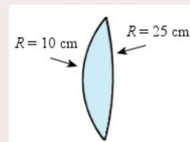
a) What is the focal length of the lens according to the thin lens formula?
