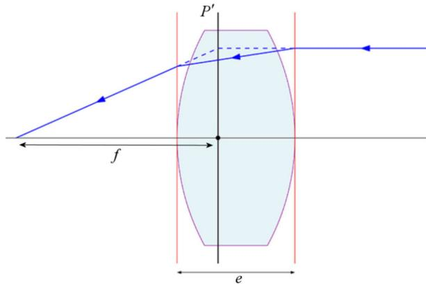
The two principal planes are not in the same place, but the focal length is the same on either side of the lens.
