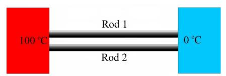
Since there are two rods, the power should be 2 times greater for the same  $\Delta T$ . Thus, with a single rod, we have
