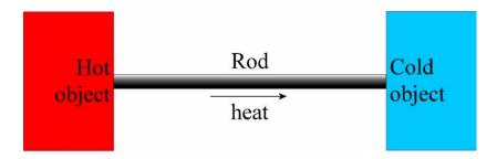
The energy that passes through the rod per second depends on the temperature difference between the ends of the rod. The greater the temperature difference, the more heat energy passes through the rod per second. So, we have
