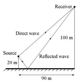
To calculate the length of the reflected path, we must realize that the length of this path is the same as for a wave going directly from the image of the source to the receiver. With the image, the length of the path can easily be calculated with a single hypotenuse.
