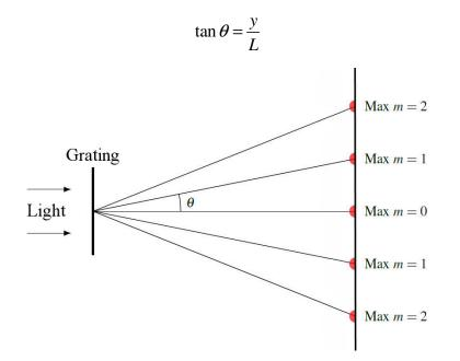
(The angle is similarly defined as the angle when there were only 2 slits. In this previous diagram,  $\theta$  is the angle of the first-order maximum.)
