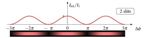
Underneath the graph, the interference pattern on a screen corresponding to this graph can be seen.
