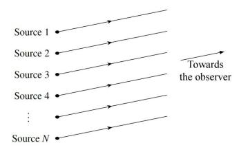
The resulting amplitude of the oscillation at a location on the screen when N waves are superimposed will now be sought.
