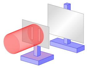
According to corpuscular theory, two bright lines should be observed on the screen. These lines are created by light particles passing through each slit.
