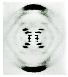
This interference pattern, obtained in 1952 by Rosalind Franklin, allowed Crick and Watson to discover the double helix structure of DNA.
