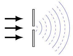
When the light from a source passes through a thin slit, the light wave spreads. (In the next chapter, this spreading of the wave when it passes through a small opening will be considered with more details.) If the light passes through two thin slits, then the waves from each of the slits are superimposed. The situation shown on the diagram on the right is then obtained.
