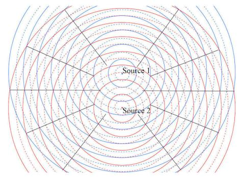
At the locations where there is destructive interference, the maxima of one the waves (circles with full lines) are superimposed with the minima of the other wave (dotted circles) so that the resulting amplitude vanishes. Along these lines, there is destructive interference.
