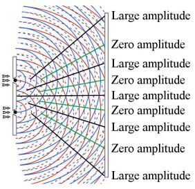
When the amplitude is great, the intensity of the light is great. Areas where the intensity is great are called *Bright fringes*. When the amplitude is zero, the light intensity is zero. Areas where the intensity is zero are called *Dark fringes*.
