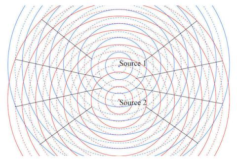
Thus, the result of the addition of 2 waves varies from one place to the other. In some places, there is constructive interference and in some other places, there is destructive interference.
