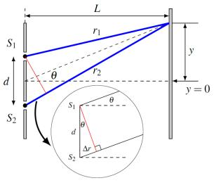
distance of the screen (L) is much greater than the distance between the slits (d).
