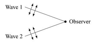
In this case, the same thing happens as with longitudinal waves: If the angle between the two sources is not too great, the results for the conditions of constructive and destructive interference remain valid and the formula of the amplitude of the resulting wave becomes an approximation.
