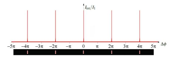
The following interference pattern was obtained with a grating comprising nearly 1000 slits (however, the laser was too thin to pass through all these slits, it passed through about a hundred slits.)
