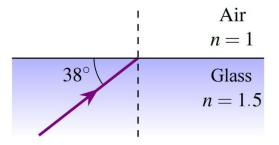
21.Light arrives at an interface between glass and air as shown in the diagram. Will the light make a total reflection or not?
