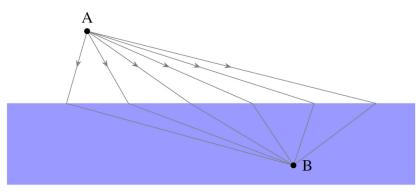
To find the fastest path, let first assume that the ray of light enters the second medium at a horizontal distance x from point A.
