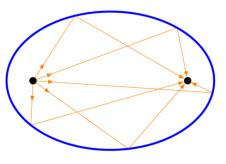
Similarly, the Paris metro was built on the same principle: passengers on a platform can hear their fellow passengers perfectly on the opposite platform. They are both located in the focii of the ellipse, which is the shape of the tunnel vault.
