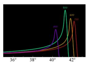
red light, the intensity is maximum when there are 42.4° (the refractive index is 1.3311) between the initial direction of the rays and the emerging ray (angle  $\phi$  in the diagram). For blue light, the angle is 40.6° (the refractive index is 1.3435). The following graph of light intensity as a function of the angle of deflection shows the difference according to the wavelength.
