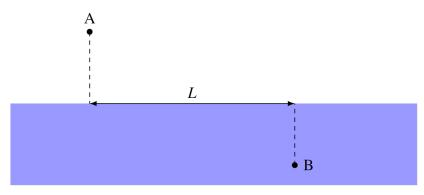
It will now be shown that the path followed by a ray of light according to the law of refraction is the one that requires the least time to travel from A to B.
