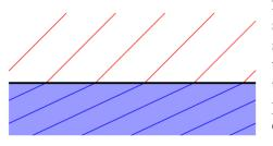
$2^{nd}$  medium travels forward less quickly than the side which is in the first medium. Therefore, this side which travels at a lower speed lags compared to the other side, and this changes the orientation of the wavefront. Since the direction of propagation is perpendicular to the wavefront, this changes the direction of propagation of the wave.
