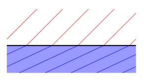
This deviation is also a refraction because it is similar to what happens when light passes from one medium to another. When the wavefront in air enters into water, its speed decreases. The part of the wavefront still in air then overtakes the part of the wave in water, and this changes the orientation of the wavefront and the direction of propagation of the wave.
