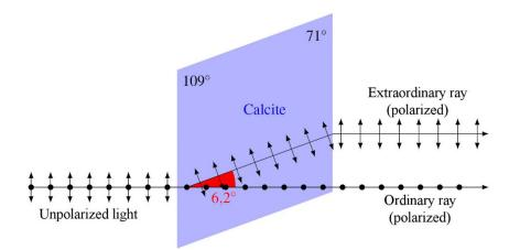
If unpolarized light passes through such a crystal, then the ordinary ray and the extraordinary ray are present at the same time. Unpolarized light is thus separated into two polarized rays with the same intensity.
