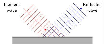
Here, the wave will not be followed with the wavefronts. Its displacement of the wave will be followed with lines showing the direction of propagation of the wave, i.e. the rays. With rays, a reflection is represented as in the following diagram.
