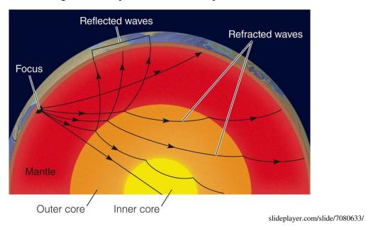
By measuring waves that arrive at the surface of the Earth, the way they have been refracted can be calculated and then the internal structure of the Earth can be inferred.
