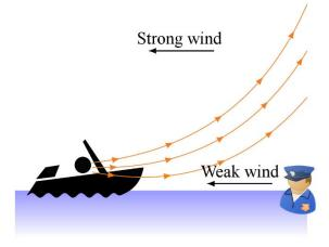
If the temperature of the air gets lower with altitude, the deviation of the sound is directed upwards instead. In this image, the person does not even hear the noise of the car since the sound is deflected and pass over his head. This is what is occurring at the surface of a lake at night when the lake is warmer than the air. You can have a big party on the lake, and nobody hears you around the lake...
