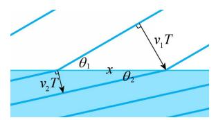
Now, the change in orientation of the wave will be calculated. During a period, the wave travels a distance vT, which is also equal to the wavelength. Since the speed is smaller in the second medium, the wave travels a smaller distance in the second medium, which means that the wavelength is smaller in the  $2^{nd}$  medium.
