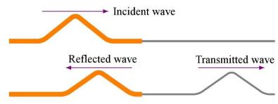
The amplitude of the transmitted and reflected waves depends on the impedance of the media. If the initial wave has an amplitude A, then the amplitude of the reflected and transmitted waves are as follows.
