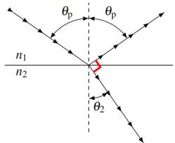
In short, there must be  $90^\circ$  between the reflected ray and the refracted ray to have a
