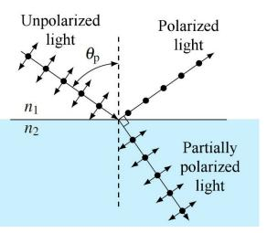
than the other. The polarization that can be reflected has lost some of its intensity to the reflection and less intensity is left for the refracted ray compared to the polarization that is only refracted. This is how polarized light can be obtained from unpolarized light with a reflection.
