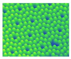
The precision is quite remarkable as the following picture shows. This image represents a silicon surface. The green dots are silicon atoms. A missing atom in the structure can be noticed at the bottom right of the picture.
