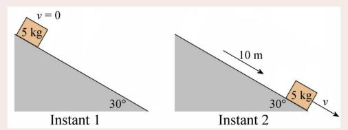
The work-energy theorem will be applied here for the motion between these two instants:
