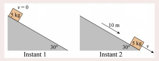
To find the work done by the forces, the forces acting on the box must be found first. There are 3 forces acting on the 5 kg box.
