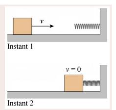
At instant 1, the spring is not compressed. Therefore, x = 0 m.
