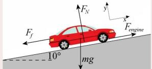
Since the car is moving at the same speed as it was on the horizontal surface, the frictional force is the same (402.8 N). The equation now becomes
