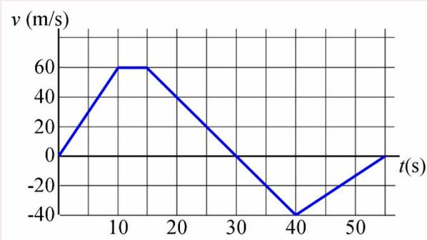
$$\begin{aligned} a &= \frac{0 \frac{m}{s} - 60 \frac{m}{s}}{30s - 15s} \\ &= -4 \frac{m}{s^2} \end{aligned}$$
